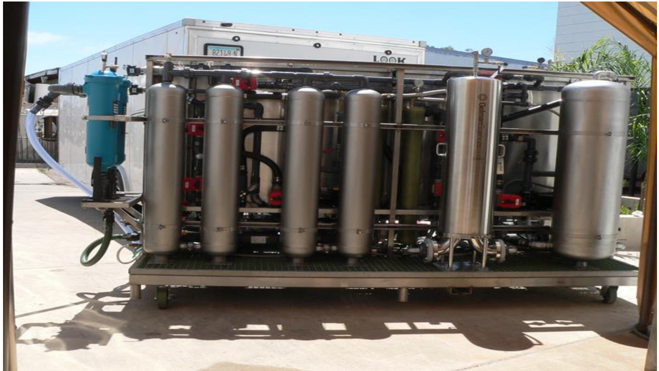
CWS fully automated skid mounted demo unit showing Vertical Membrane Technology (above) and PLC Assembly (below). Unit is capable of treating 100,000 gallons per day.
